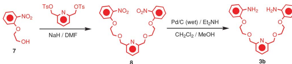
Scheme 3 Synthesis of the diamine compound 3b through an intermediate compound 8 .
